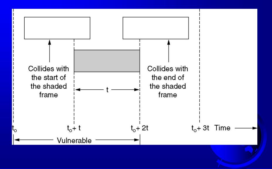
Analysis of Pure ALOHA (cont.) Probability k frames generated per frame time  $G^k e^{-G}$  $\Pr[k] = \cdots$ k! $Pr[0] = e^{-G}$  $\sim$  Need two frame times empty, 2G generated - for two slots,  $Pr[0] = e^{-2G}$  $\sim$  Using S=GP<sub>0</sub>, throughput per frame time  $S = Ge^{-2G}$
