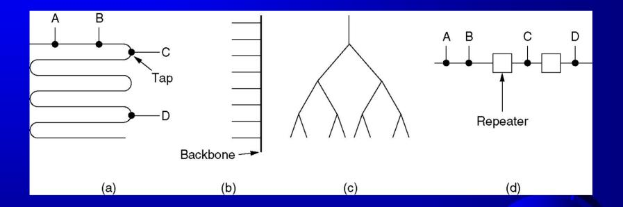
Cable topologies. (a) Linear, (b) Spine, (c) Tree, (d) Segmented. Repeaters?
