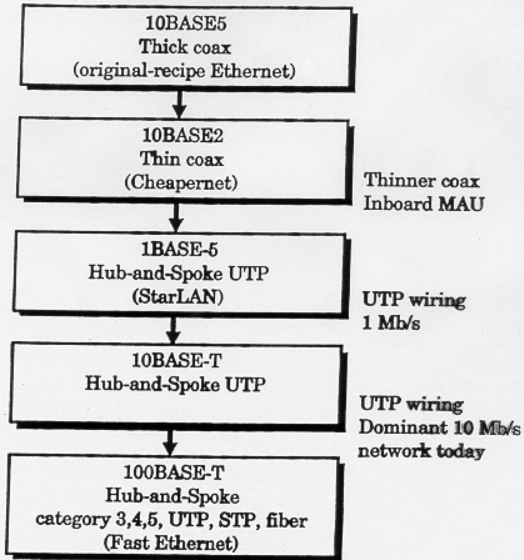
Figure 1.4 Lineage of Fast Ethernet
