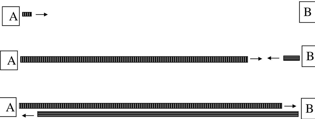
B begins to transmit at  $t = t_{prop} - \delta$ ; B detects collision at  $t = t_{prop}$
