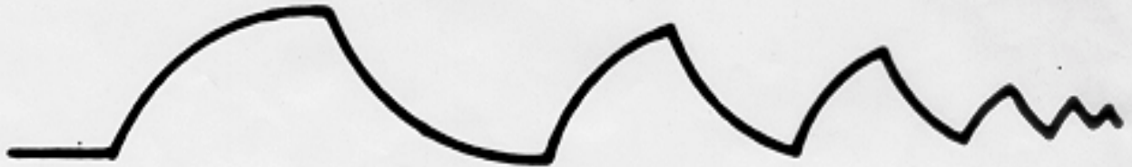
FIGURE 2.1 Attenuation of Digital Signals
