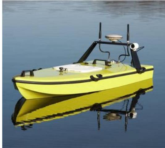
Figure 4.9. CEE-USV Unmanned Sonar (CEE-USV | CEE Hydrosystems, n.d.)
