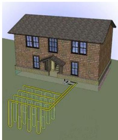
**Figure 2.9: Schematic of typical ground source heat recovery system (National Park Service 2010).**
