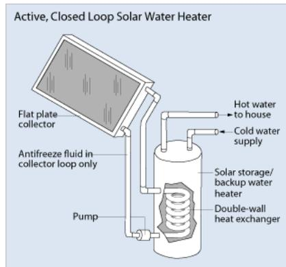
**Figure 2.5: Active, closed loop solar hot water system (US Dept. of Energy, 2009)**
