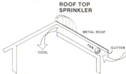
**Figure 2.1: Roof top sprinkler, integrated conductive and evaporative cooling (Western Solar Utilization Network, 2010).**
