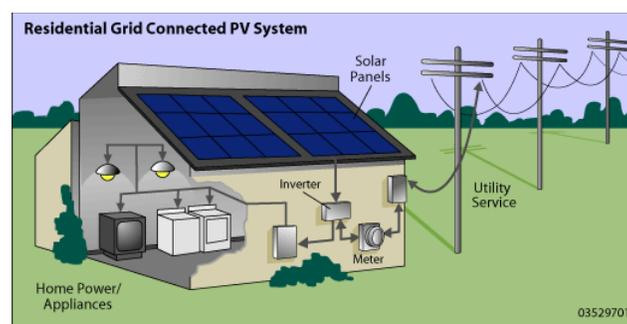
**Figure 2.2: Grid connected photovoltaic system (US Dept. of Energy, 2009).**
