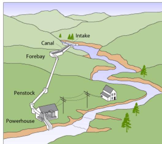
**Figure 2.8: Typical Construction of a Run of the River Hydroelectric Power System (US Dept. of Energy, 2009).**
