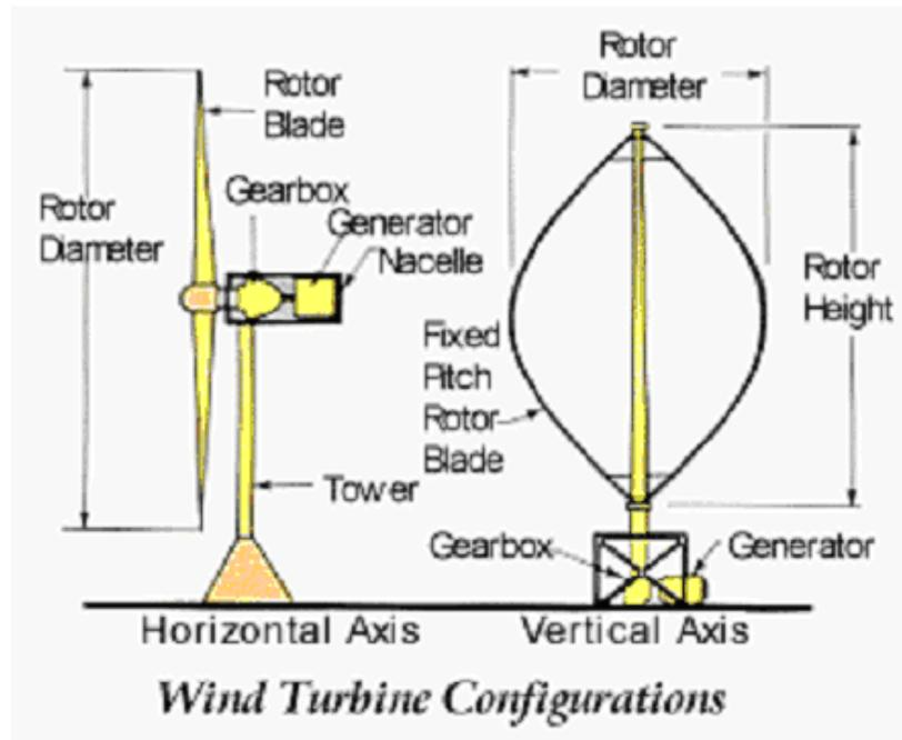
**Figure 2.7: Comparison of a vertical axis and horizontal axis wind turbine (85 Twenty First Century Energy 2010).**
