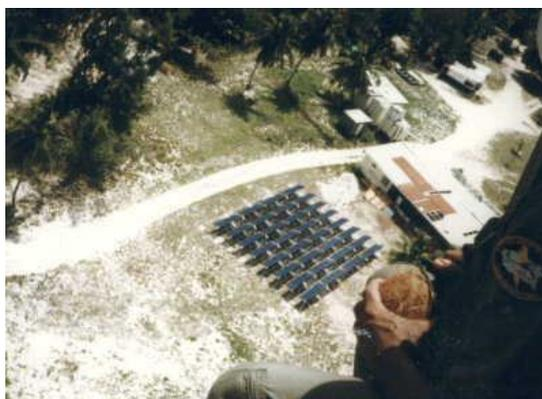
**Figure 2.4: 15 kW photovoltaic system on Mona Island, Puerto Rico (Bing, 1998)**
