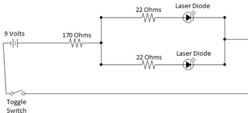
FIGURE 11: CIRCUIT DIAGRAM
