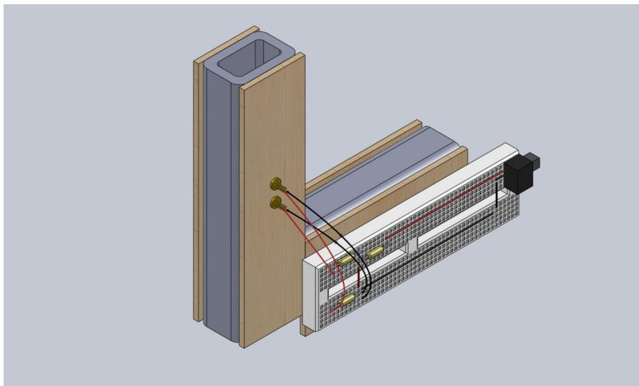
FIGURE 13: COMPLETE WIRING FOR EMITTER CIRCUIT
