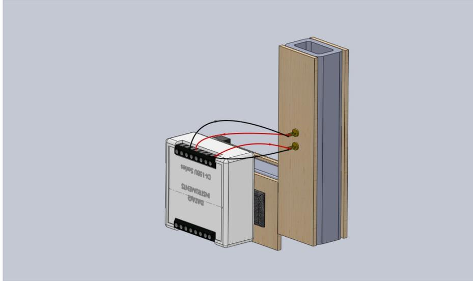
**FIGURE 15: COMPLETE WIRING FOR RECEIVER CIRCUIT**
