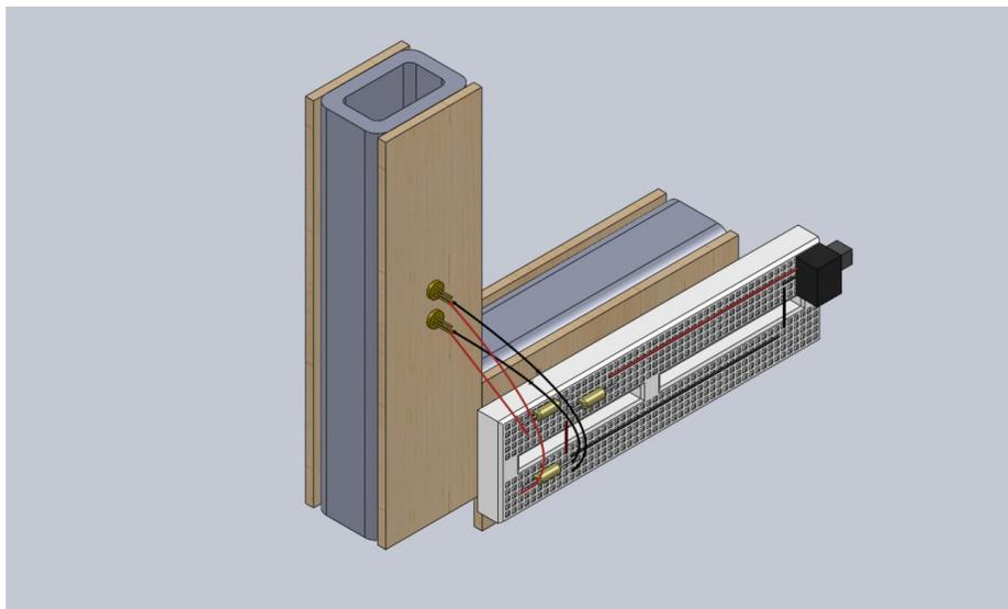
FIGURE 13: COMPLETE WIRING FOR EMITTER CIRCUIT
