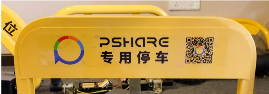
Figure 26: PShare lock with QR code for smartphone pairing
