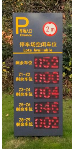
Figure 17: Huawei parking complex entrance with digital display for available parking spaces
