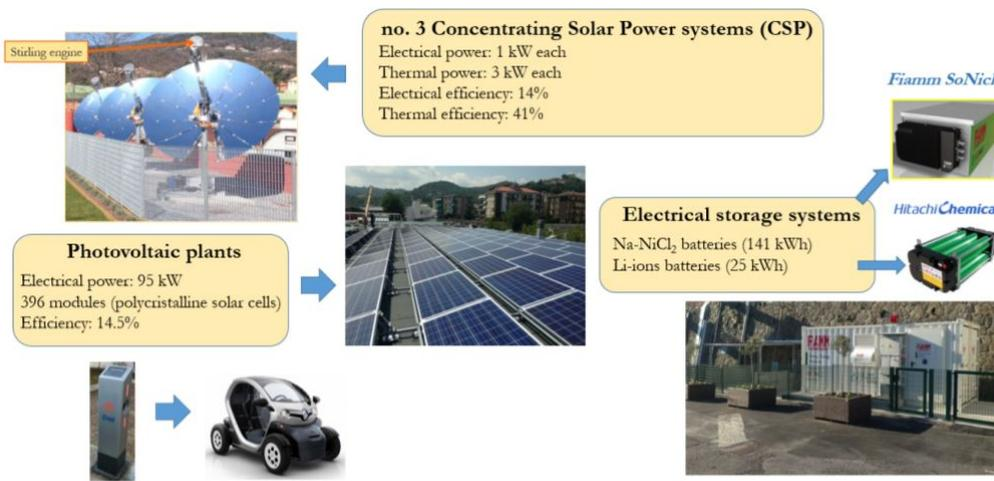
Figure 3: Smart Polygeneration Microgrid at Genoa University (Brenna et al., 2016).
