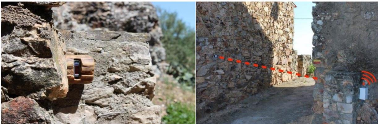
**Figure 2.6: Installed Light Beam Sensor in Naturtejo National Park (Dionisio, 2016).**
