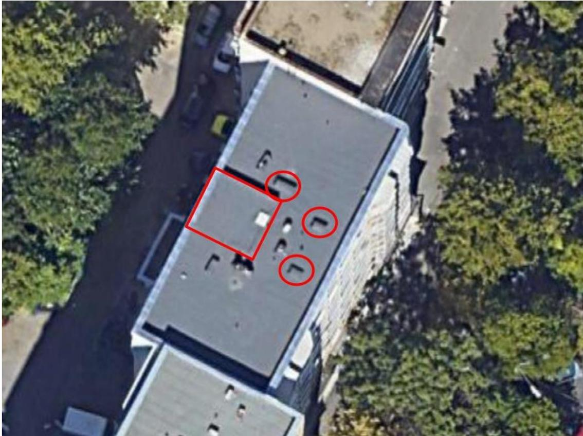
*Figure 3.5: Double orientation building, the red square indicates elevator shaft, the red circles indicate the sewer pipes*
