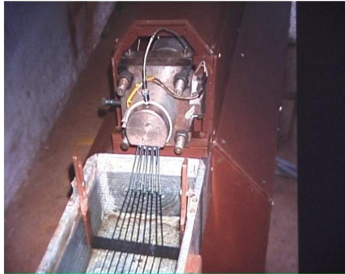
Figure 14: Example of Pelletizer Machine in India (Van Den Berg, 2009)
