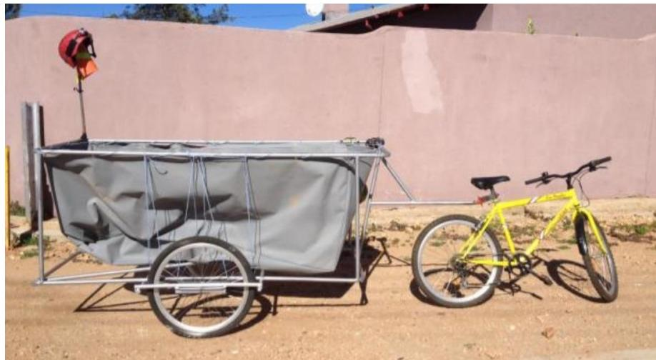
Figure 9: Completed Recycle by Bicycle Prototype (Jacobsen et al., 2014)
