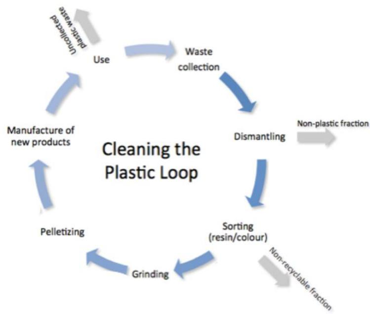
Figure 13: Plastic Recycling Process (adapted from Haarman, 2015)
