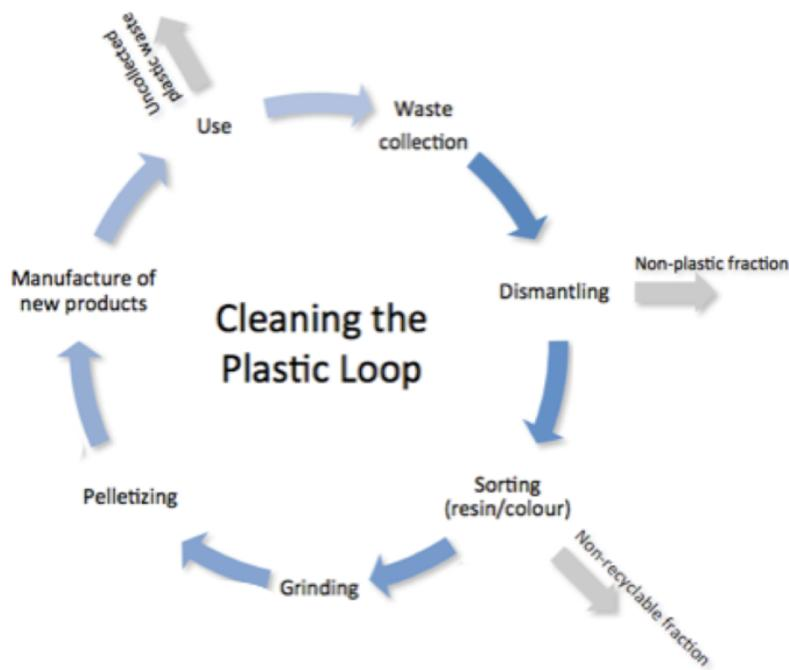
Figure 15: Plastic recycling process (adapted from Haarman, 2015)
