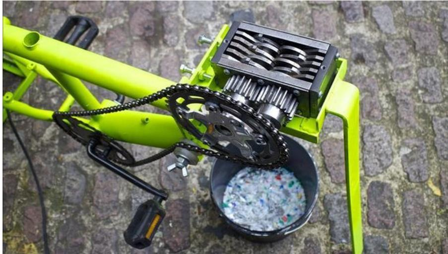
Figure 27: "The Ingenio" bicycle-powered plastic shredder (Holaciudad, 2013)
