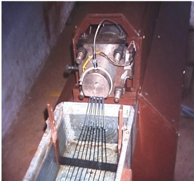
Figure 16: Example of pelletizer machine in India (Van Den Berg, 2009)
