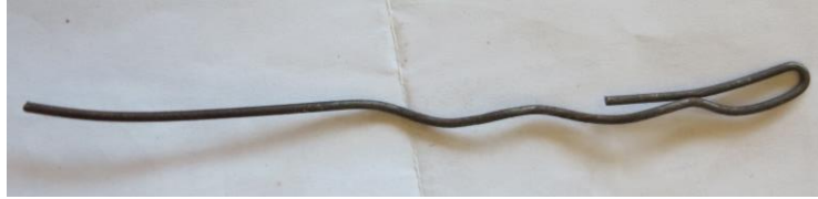
Figure 28. Needle Tool Used for Weaving Tire Chair
