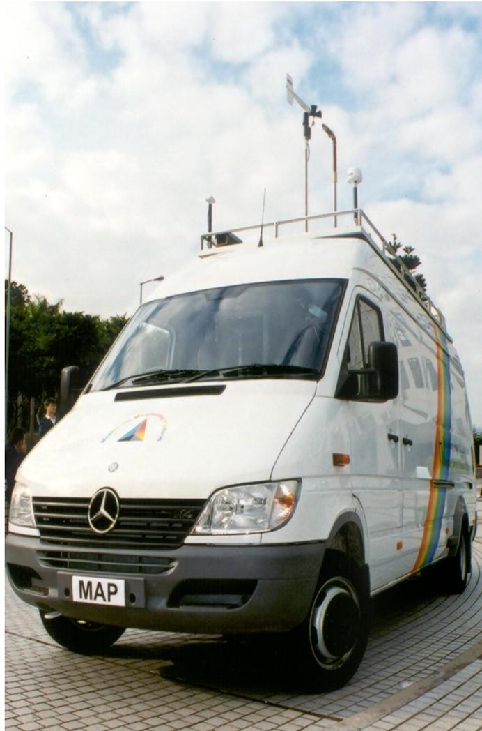
Figure 0-1: Mobile Real-time Air Monitoring Platform
