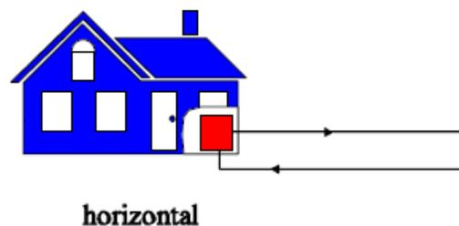
**Figure 2.12(b): Horizontal Closed Loop**
