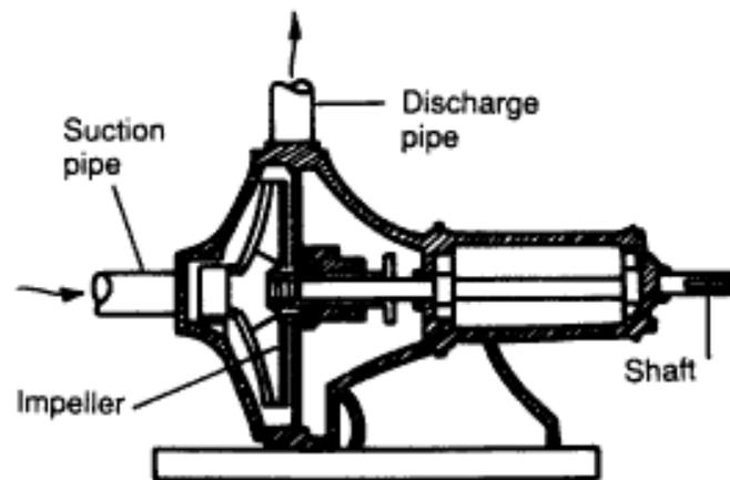
Figure 2.1: Centrifugal Pump Cross Section (Scherer, 1993)
