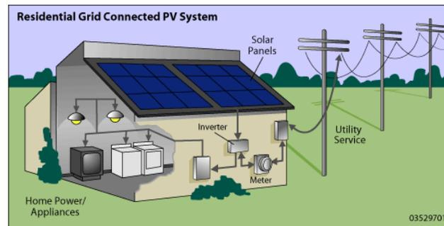
**Figure 2.5: Grid Connected Photovoltaic System (Department of Energy, 2009)**
