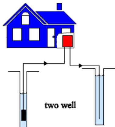
**Figure 2.13: Two Well Open Loop System**
