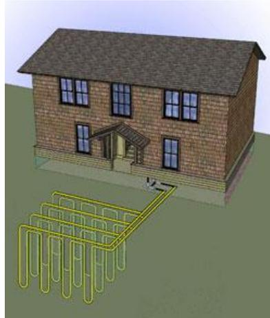
**Figure 2.14: Schematic of Curry Village Ground Source Heat Recovery System
