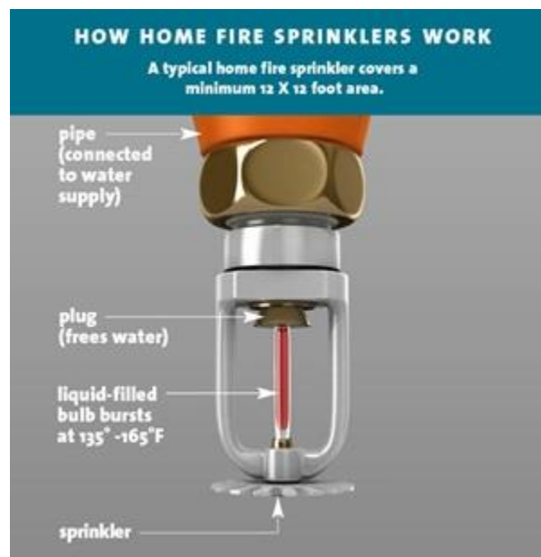
Figure 2: How Home Fire Sprinklers Work (NFPA, N.d.).
