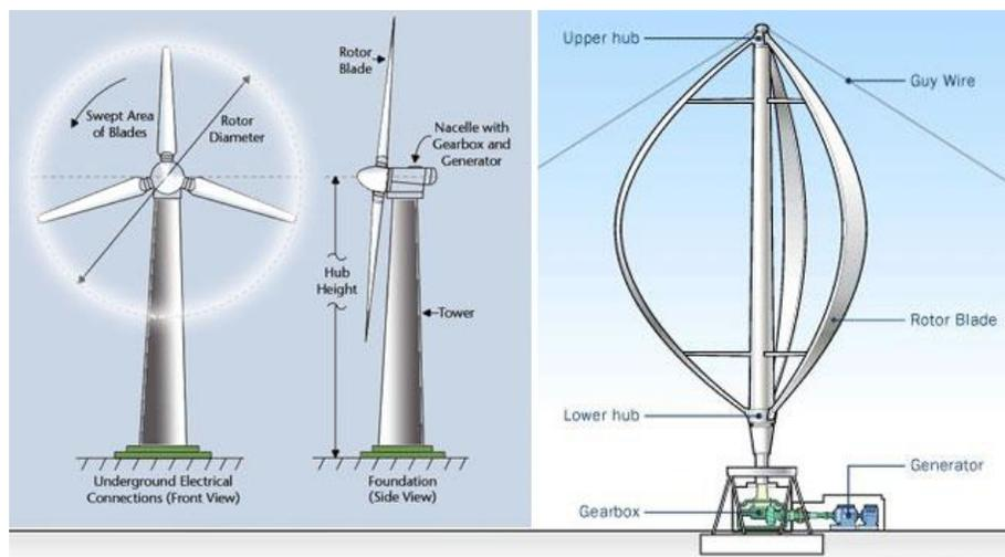
Figure 2. 5. 1: Comparison of Vertical (right) and Horizontal (left) Wind Turbines (Eco Energy, n.d.)
