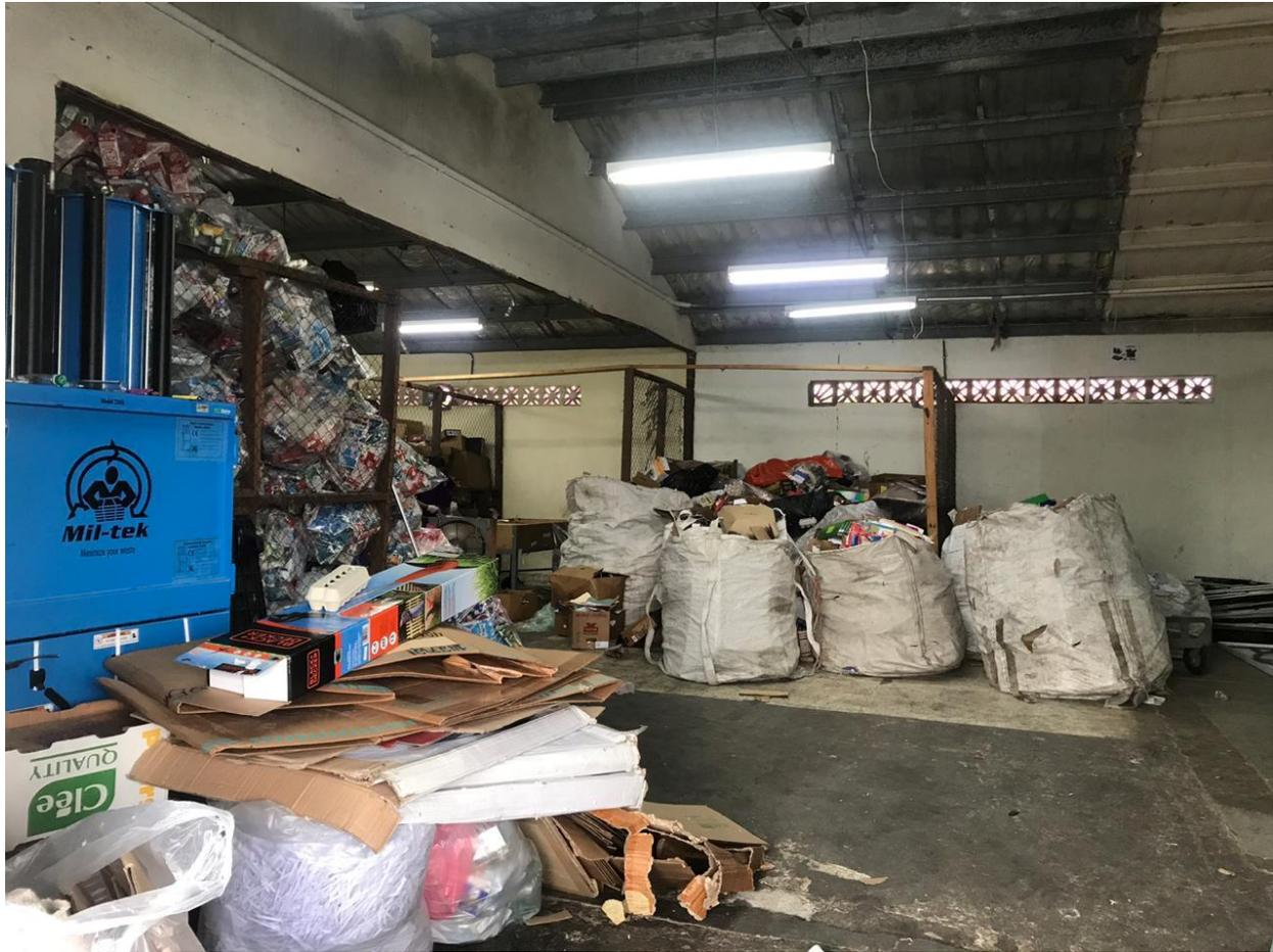
*Figure 10: The baler (left), the sorting sacks, and the storage cages at CAR (FAS Panama, 2019)*
