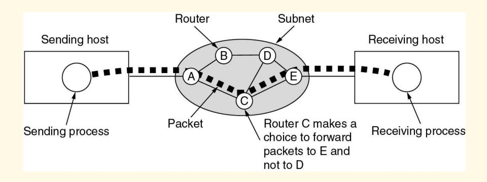
End-to-end delay includes multiple hop link delays.
