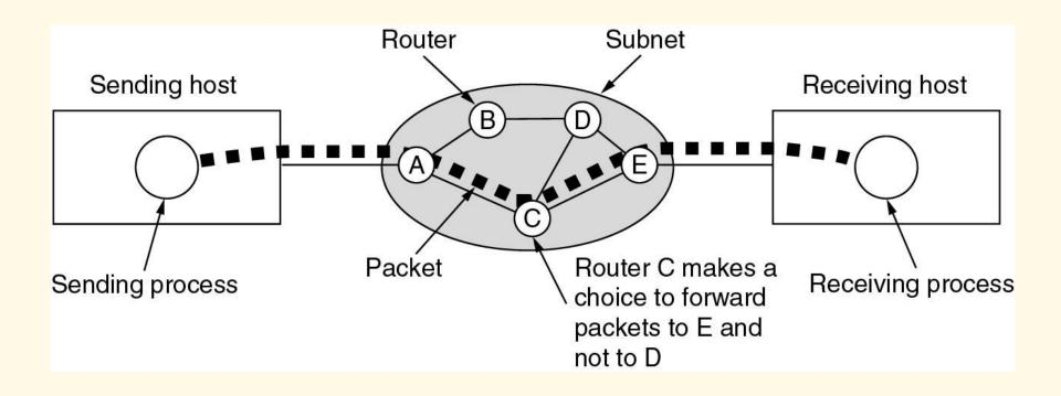
End-to-end delay includes multiple hop link delays.
