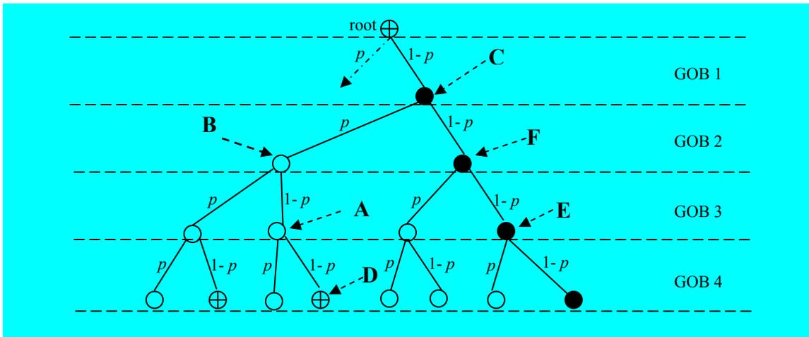
**Figure 4.3.** Binary tree for the possible decoded versions of a GOB using Intra Update
