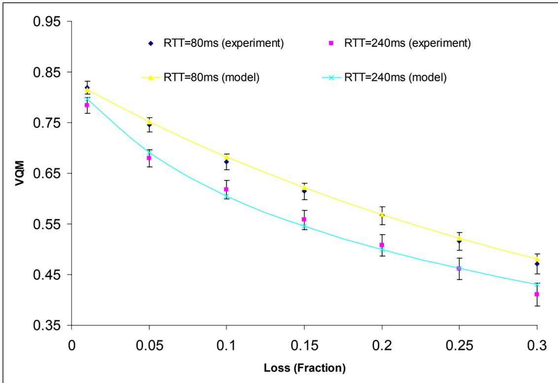
Figure 6.12 VQM vs. loss with RPS NACK (video clip: Coastguard)
