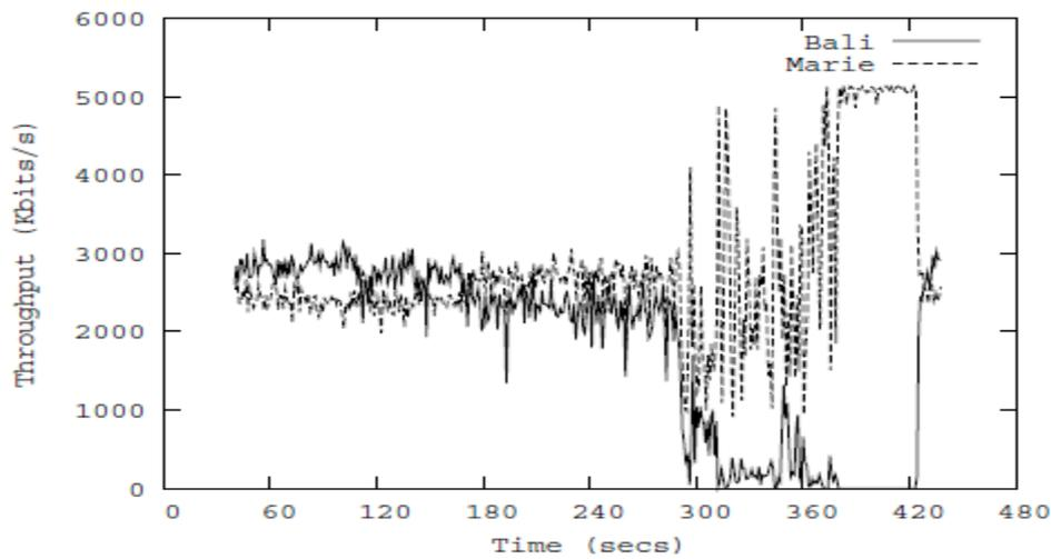
Fig. 11. Measured throughput in Mb/s for two hosts (one mobile), TCP traffic
