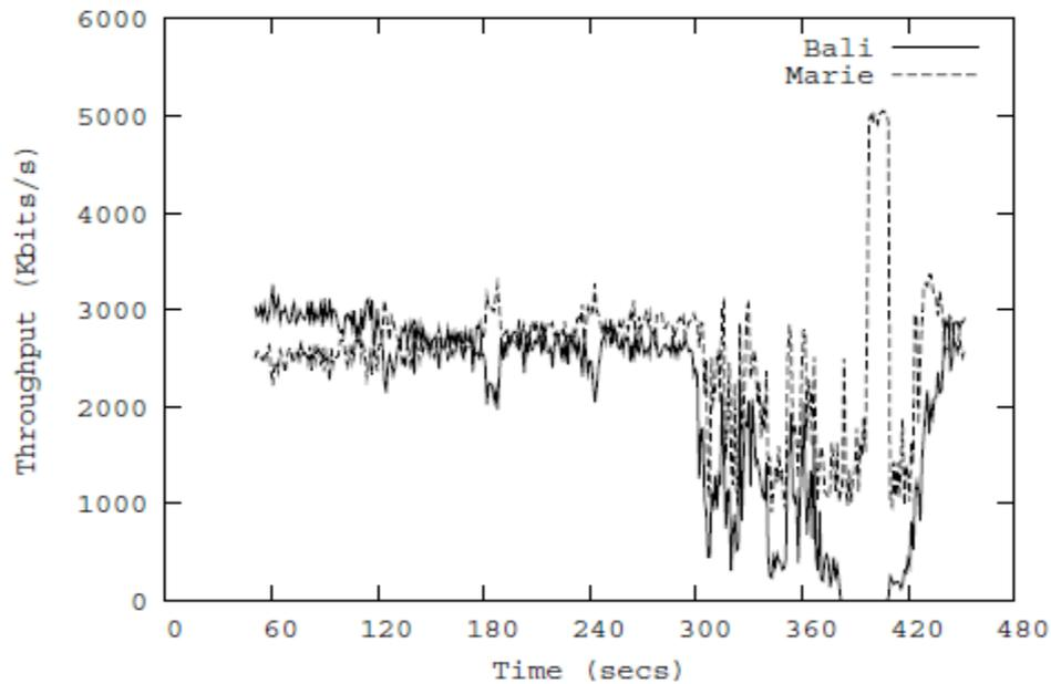
Fig. 13. Measured throughput in Mb/s for two hosts (one mobile), UDP traffic
