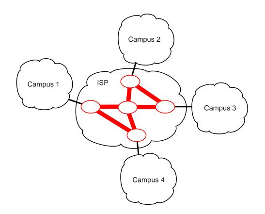
**Example:** Multiple campuses connected to a common ISP by low-speed tails.
