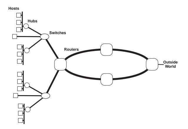
**Example:** The elements of a campus network have very different capabilities. If resources are not assigned to a path you can account for hardware realities and put the tagging/shaping/policing machinery only where you need it).
