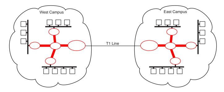
**Example:** Two campuses connected by a low-speed WAN link.
