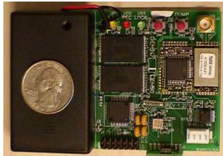
Figure 3: The Berkeley GPSADXL fall sensor
