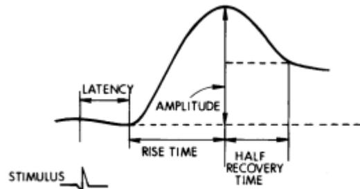
Figure 5. Graphical representation of principal EDA components.
