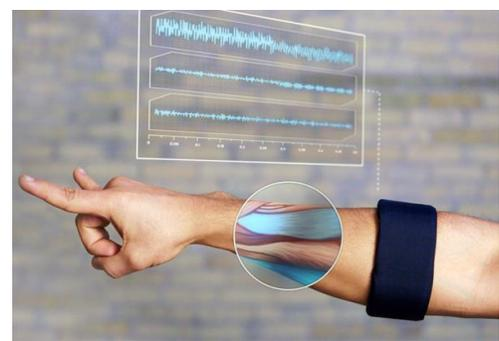
armband worn below the elbow that measures EMG can be detect various gestures from your fingers, thereby enabling gesture-based interaction with computers and video games, or perhaps interaction with your home like switching on/off light bulbs by flicking your fingers.
