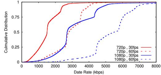
Figure 9: Encoding Rates for Video with Different Frame Rates
