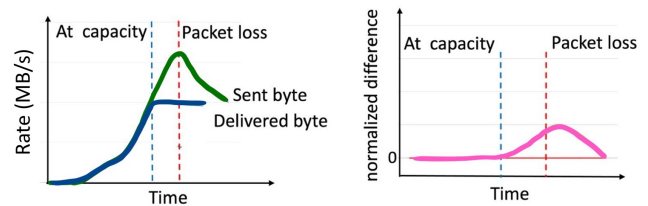
Fig. 1: SEARCH: (left) sent and delivered rates over time, and (right) normalized difference over time.
