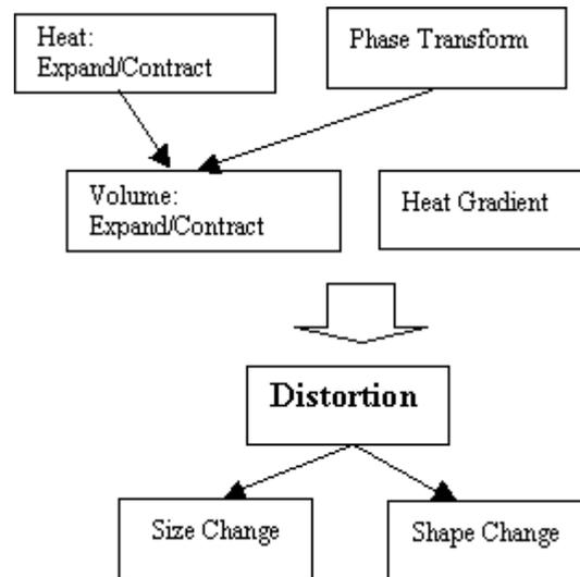
**Figure 11: Mechanism of Distortion**
