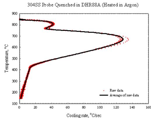
Figure 3: Cooling rate graph of a quenchant
