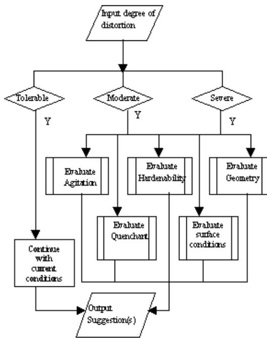
Figure 13: Flowchart for DSS (Distortion Case)
