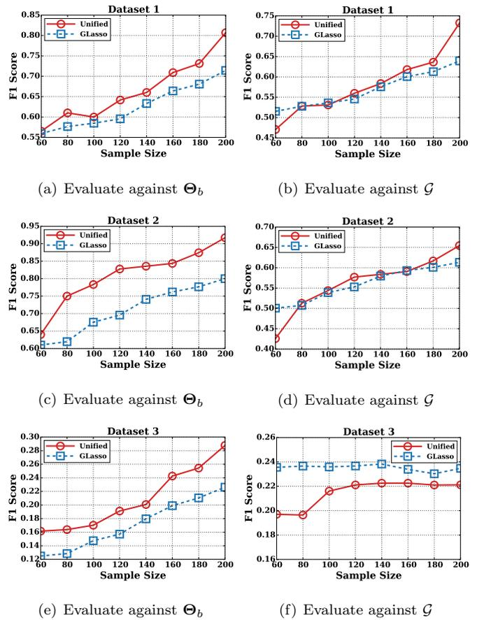
Figure 3: Comparison between UGLASSO and GLasso on three synthetic datasets in terms of F1 score on connectivity inference.
