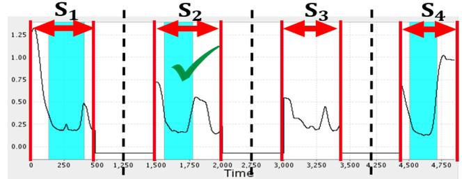
Fig. 4: This motif includes three instances of Screw. The  $S_2$  segment instance is selected as the best instance for the primitive learning algorithm based on the DTW score. (Reduction in size of blank spacer shown by dotted lines.)
