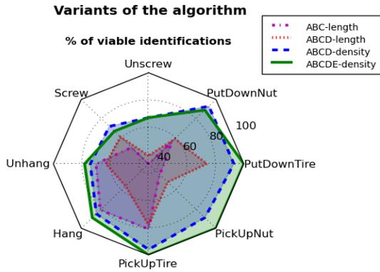
Fig. 5: Percentage of viable identifications for each primitive using different variants of the algorithm.
