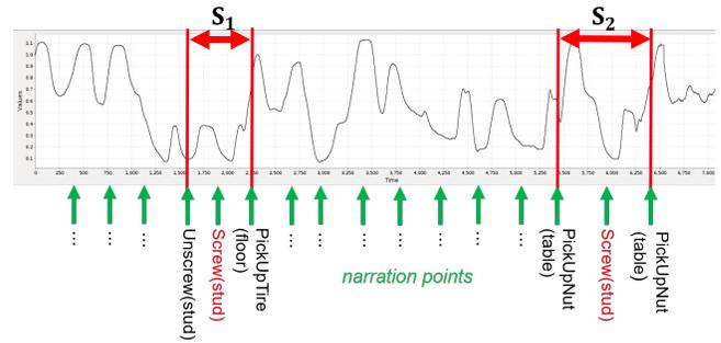
Fig. 1: Raw hand motion data with respect to a specific reference object labeled with narrations (distance from right hand and stud shown here).
