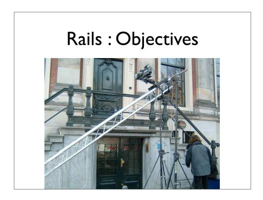
A generalization of this "camera track" idea is to borrow an idea from the film industry. One of their solutions to this problem, is to construct rails, and put the camera on a little cart, known as a Dolly, that rides on the rails.
