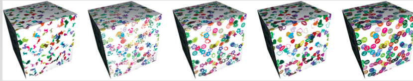
Different glyphs applied to a cube using the glyph bombing shader described in Section 10.6. (3Dlabs, Inc.)
