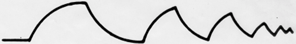
FIGURE 2.1 Attenuation of Digital Signals
