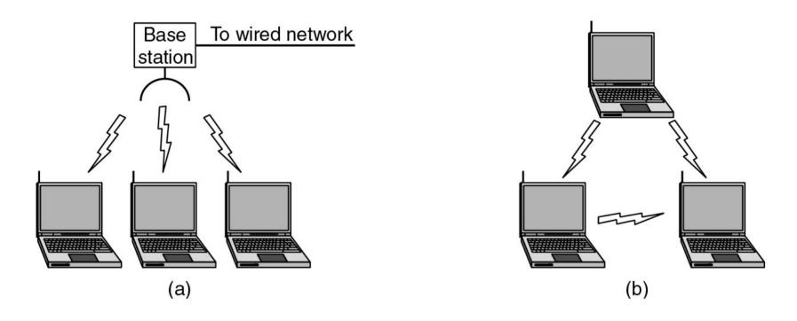
Figure 1-36.(a) Wireless networking with a base station. (b) Ad hoc networking.
