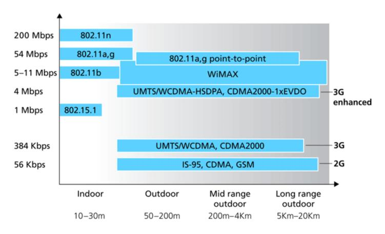
Figure 6.2 Link characteristics of selected wireless network standards
