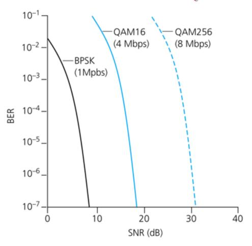
Figure 6.3 ♦ Bit error rate, transmission rate, and SNR
