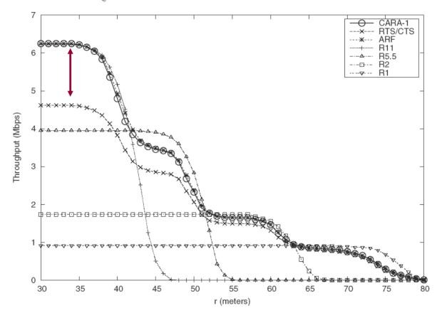
Fig. 6. Throughput comparison of our proposed rate adaptation scheme (CARA-1) against RTS/CTS, ARF, and single-rate schemes for one-to-one topology networks with various distance (r) [CARA paper]
