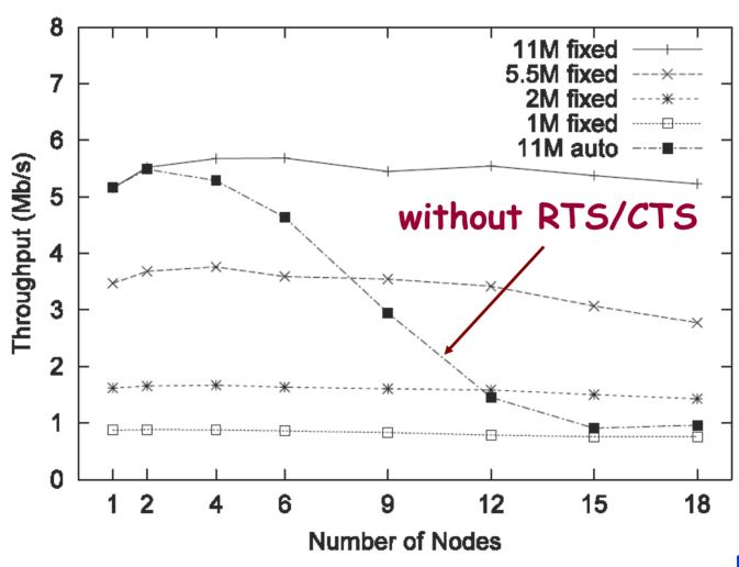
**Fig. 7** Throughputs with node contentions.
