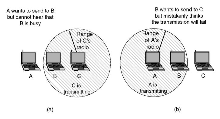
Figure 4-26.(a)The hidden terminal problem. (b) The exposed station problem.
