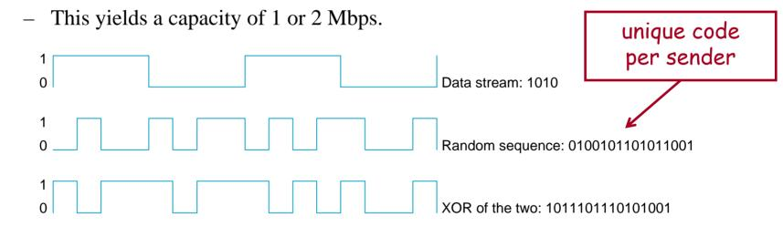
Figure 2.37 Example 4-bit chipping sequence
