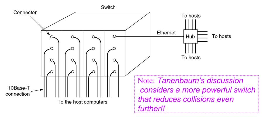
Figure 4-20.A simple example of switched Ethernet.
