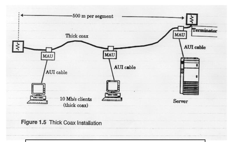
MAU device is physically hooked on main cable.
