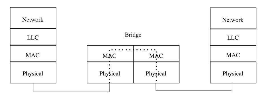
A bridge is a store and forward device that **separates** collision domains.
