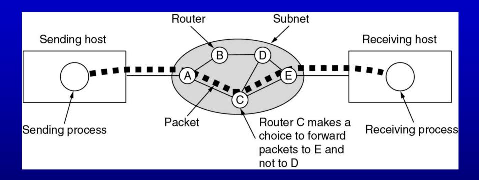
End-to-end delay includes multiple hop link delays.
