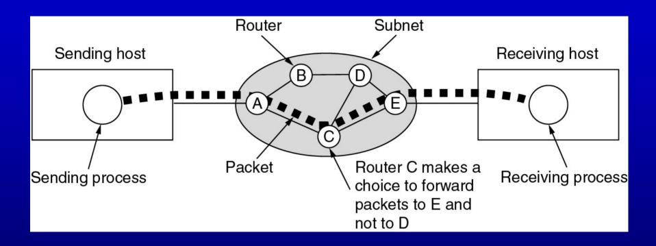
End-to-end delay includes multiple hop link delays
