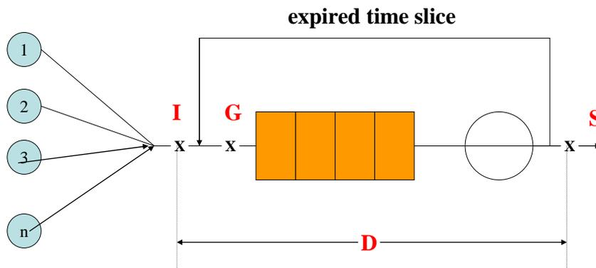
Preemptive RR is a small variant of RR designed to give priority to very short jobs. Upon the arrival of a new process at the scheduler queue, the currently running process is preempted in mid time slice. The newly arriving process then receives one initial time slice before being enqueued at the back of the scheduler queue. Once the preempting process completes, the preempted process is resumed to receive the remainder of its preempted time slice of service.
