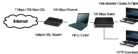
Figure 3: Case Study Network Topology
