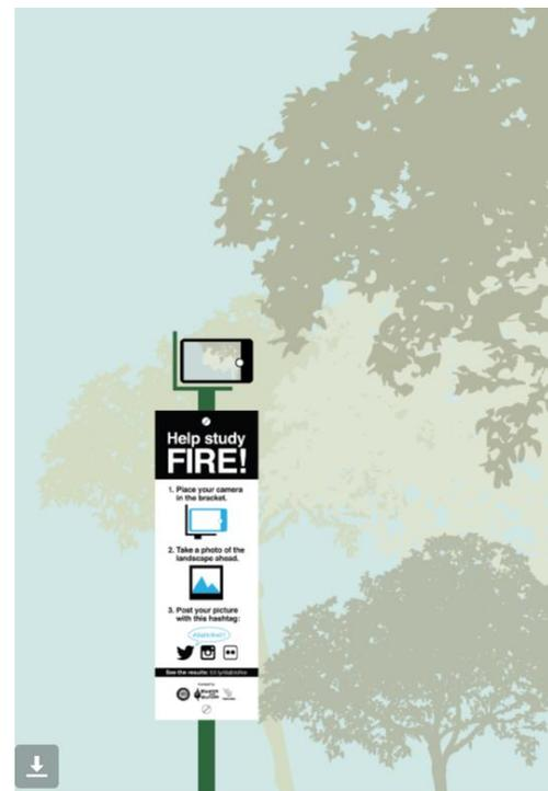
Figure 5.1: Diagram of a crowdsourcing monitoring stand (Nerds for Nature, 2015)
