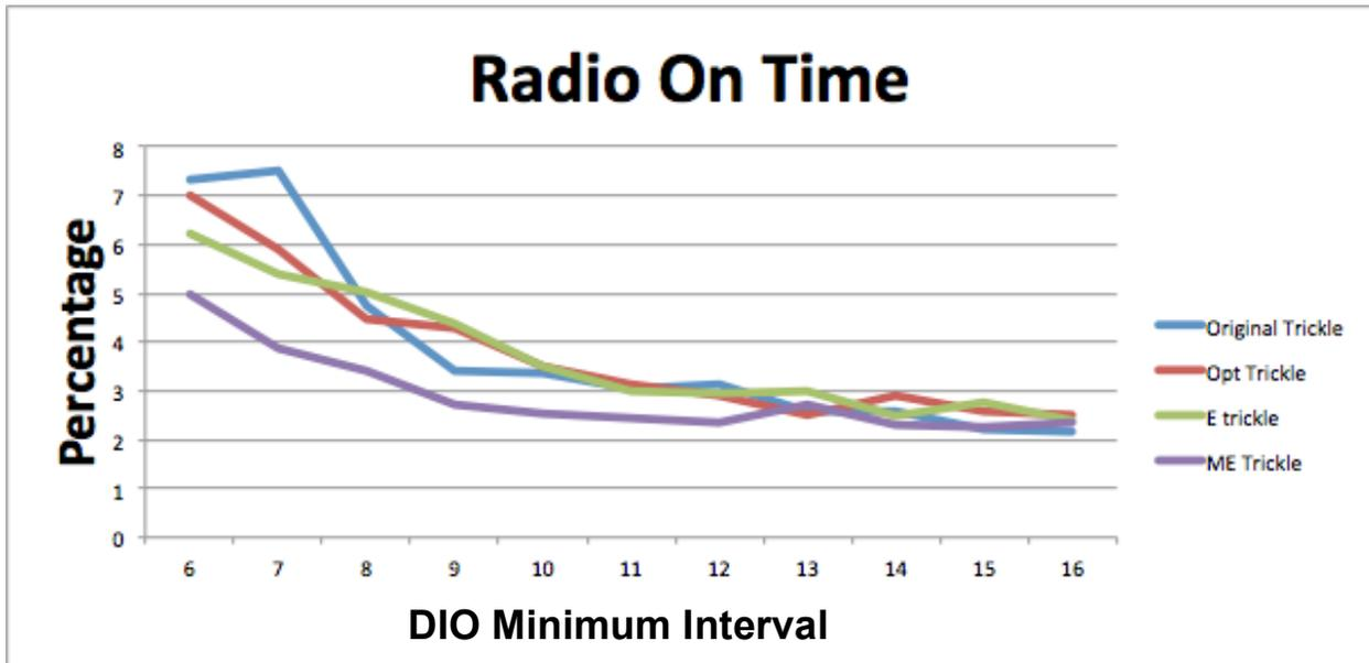
Figure 17: Radio on time versus DIO Minimum Interval
