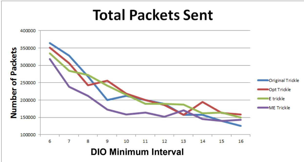
Figure 16: Total packets sent versus DIO Minimum Interval
