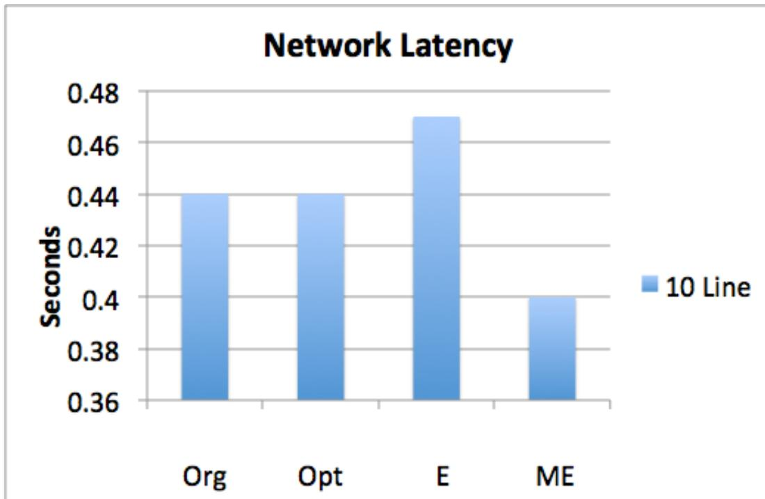
Figure 39: Network latency for 10 node line configuration
