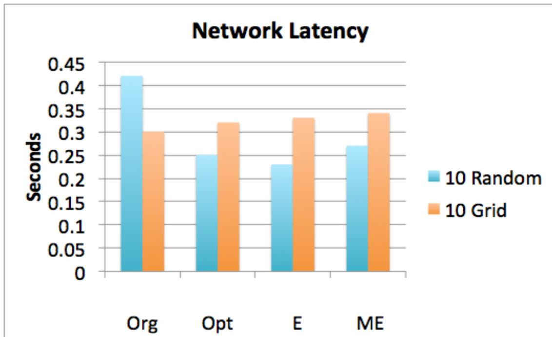
Figure 38: Network latency for 10 client node configurations
