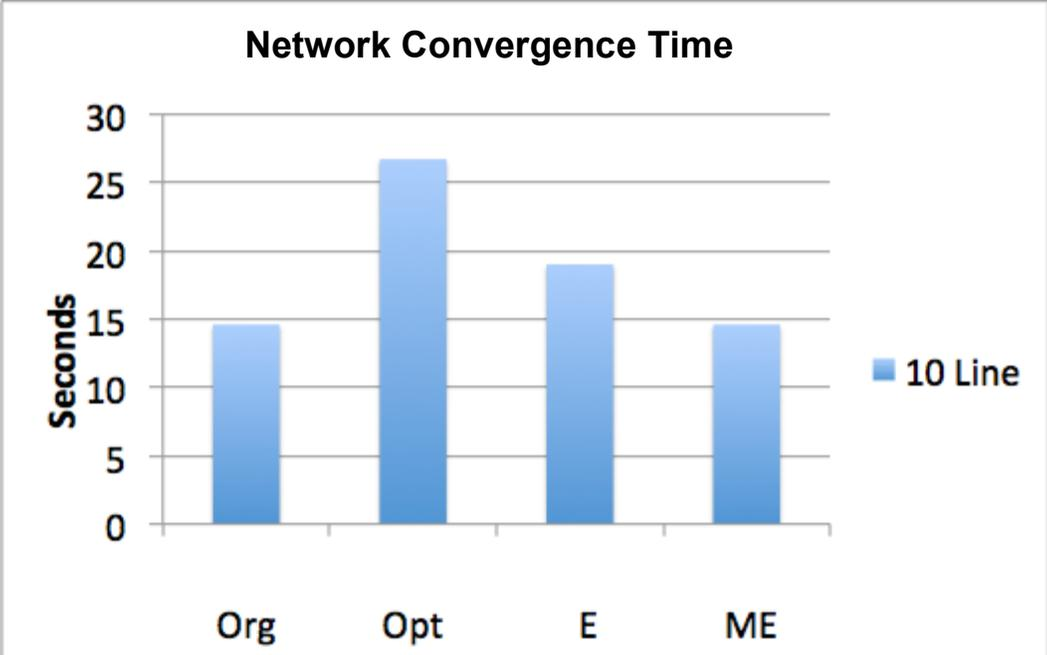
Figure 35: Network convergence time for 10 node line configuration
