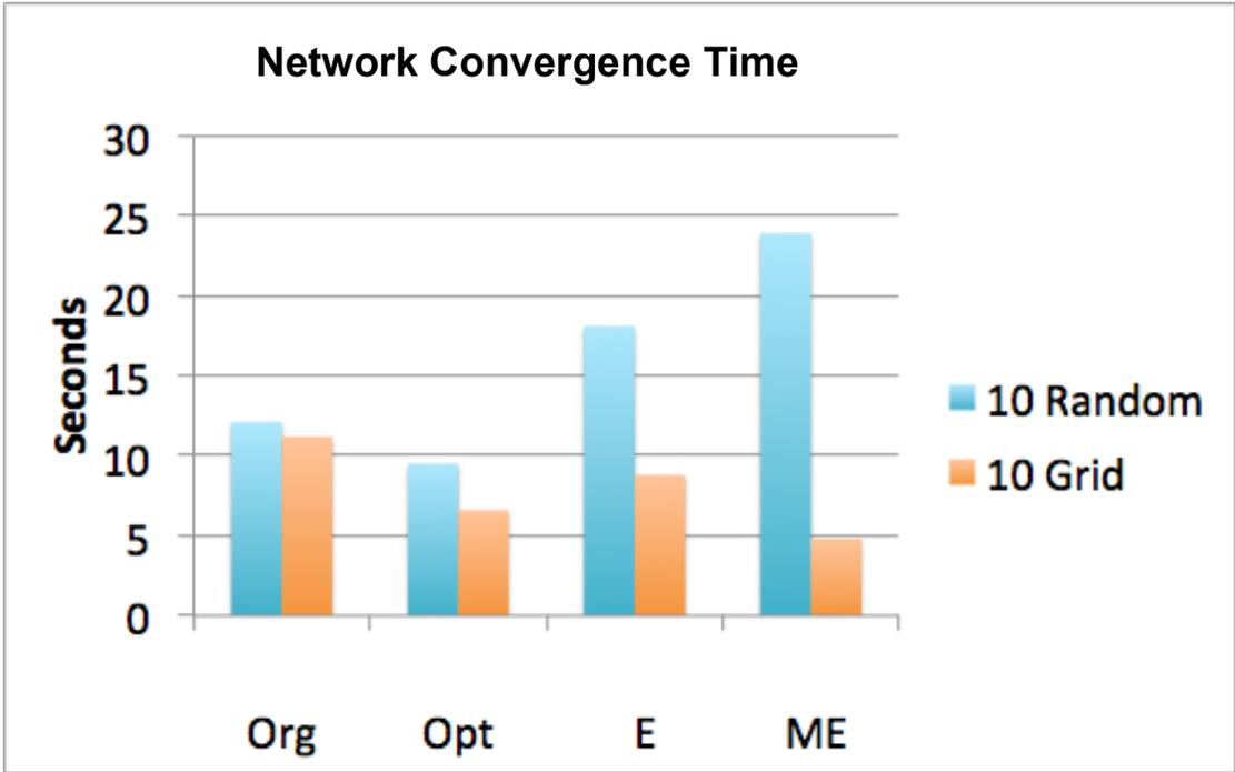
Figure 34: Network onvergence time for 10 client node configurations
