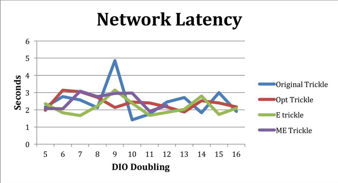
Figure 22: Network Latency versus DIO Doubling
