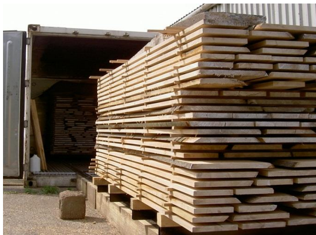
Figure 2.4- 1: Wood Stacking and Drying ( http://www.lumberbylance.com/kiln.php )
