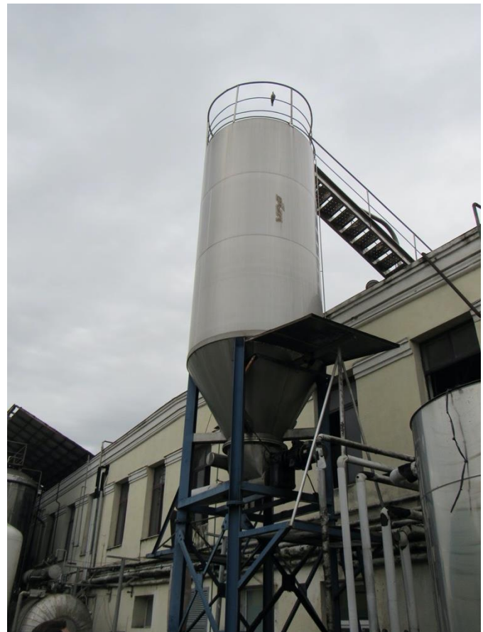
Figures 29 and 30: The spent grain silo at Birra Tirana. The left figure shows the chute used to dispense the grain into farmers' trucks. Taken on Nov. 19, 2019.
