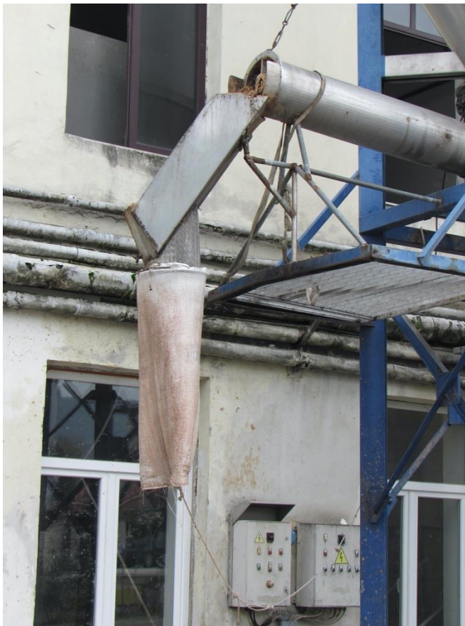
Figures 29 and 30: The spent grain silo at Birra Tirana. The left figure shows the chute used to dispense the grain into farmers' trucks. Taken on Nov. 19, 2019.
