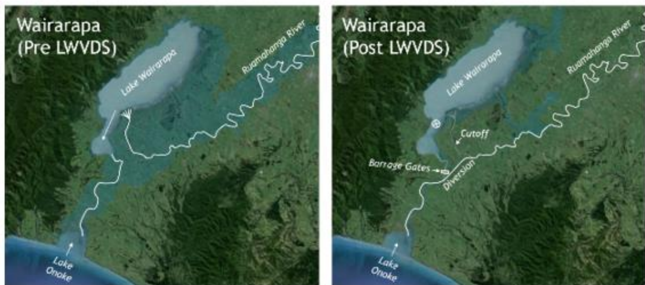
Figure 1 - The Lower Wairarapa Valley Development Scheme, which contains the diversion of the Ruamahanga straight into Lake Onoke and the Blundell Barrage Gates, dramatically reduced the extent of flooding, as shown in light blue (Google, 2015).
