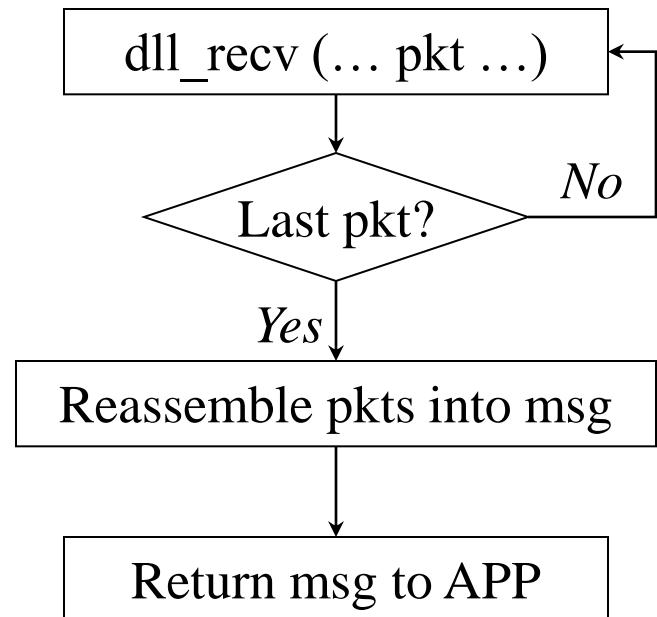
Note: you need have a mechanism to decide the last packet in a message (EOM). The diagram here offers only a reference.
