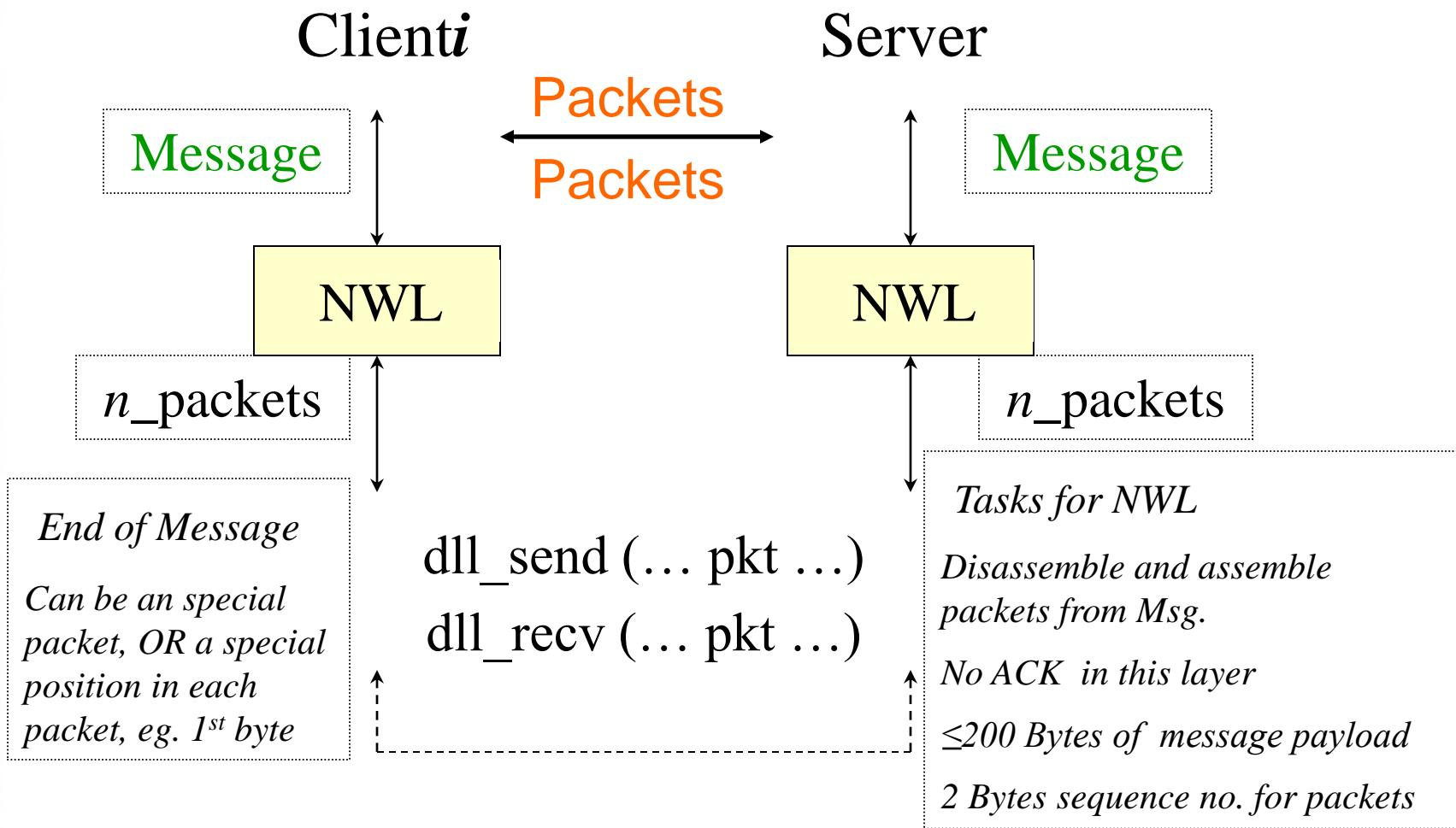
Note: The network layer will send packets until blocked by the Data Link Layer. But **HOW?**
