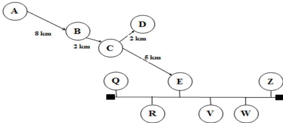
Given the internet pictured above with a propagation speed of **200 m/microsecond** on the **100BASE5 LAN** and a propagation speed of **150 m/microsecond** on the store-forward packet-switched **WAN** where nodes **Q, R, E, V, W** and **Z** are equally spaced on the **Ethernet** with nodes **Q** and **Z** at opposite extreme ends.
