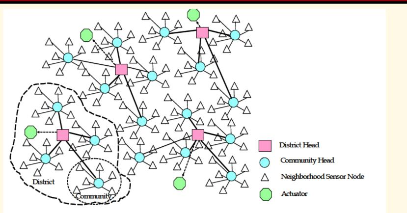
Figure 1 Hierarchical Scalable Sensor Network Architecture
