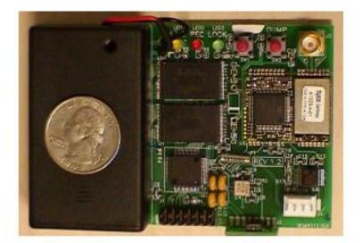
Figure 3: The Berkeley GPSADXL fall sensor
