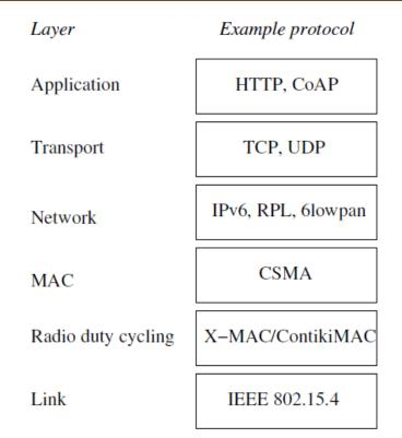
Figure 1. The low-power IPv6 stack consists of the standard IPv6 protocols at the network layer and transport layers, and of new protocols from the network layer and down.
