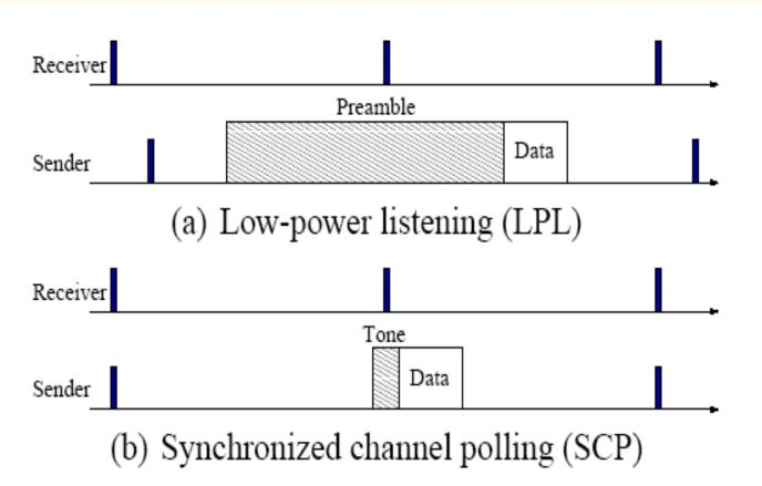
Figure 1. Sender and receiver synchronization schemes.
