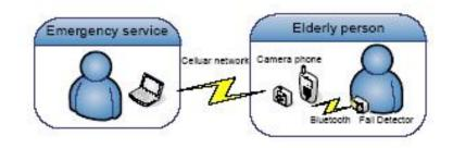
Figure 2: Fall detector system setup
