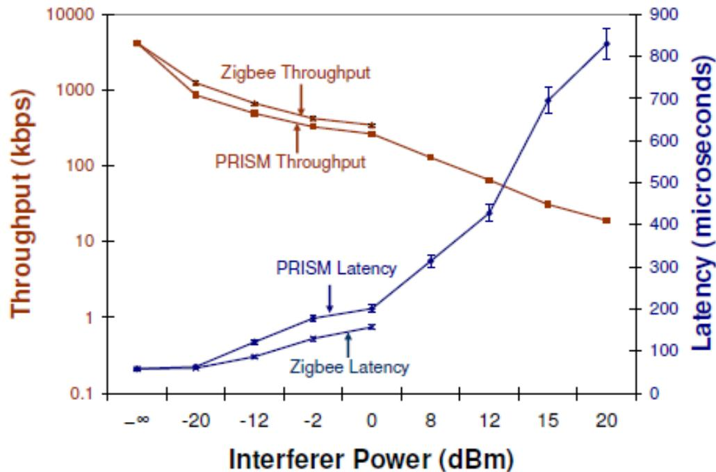
*Throughput and latency vs. interferer power caused by interference affecting dynamic range selection.*
