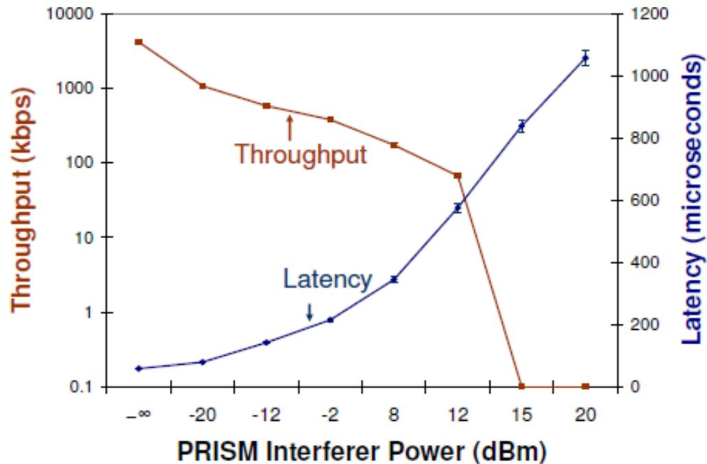
*Throughput and latency vs. interferer power caused by interference affecting timing recovery.*
