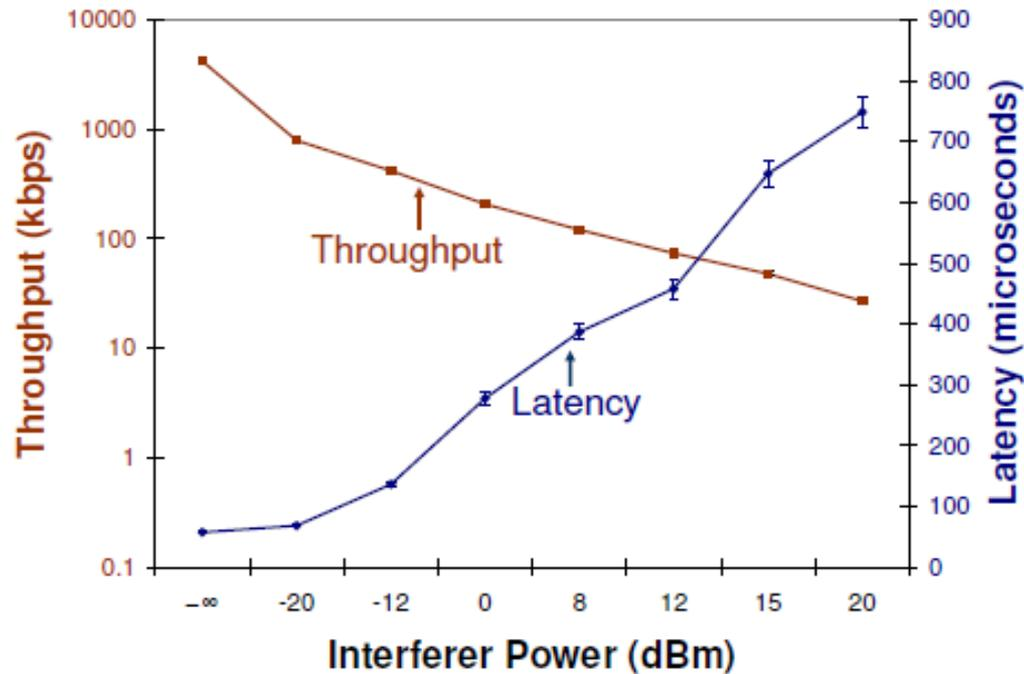
*Throughput and latency vs. interferer power caused by interference affecting header processing.*
