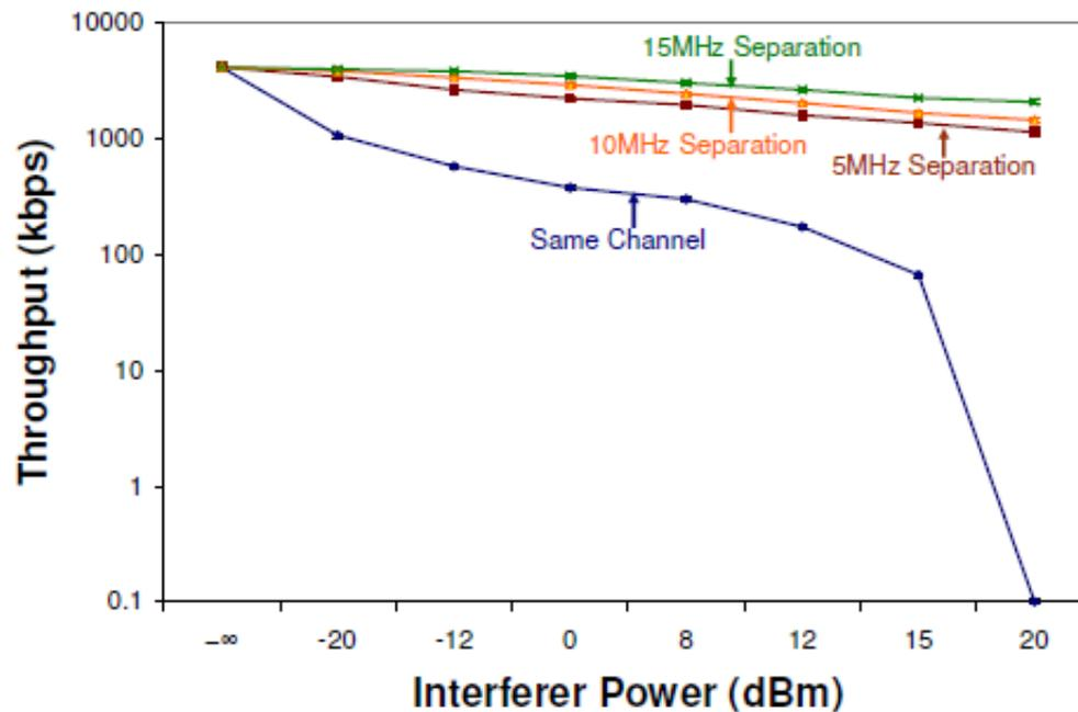
*Throughput and latency vs. interferer power with frequency separation.*
