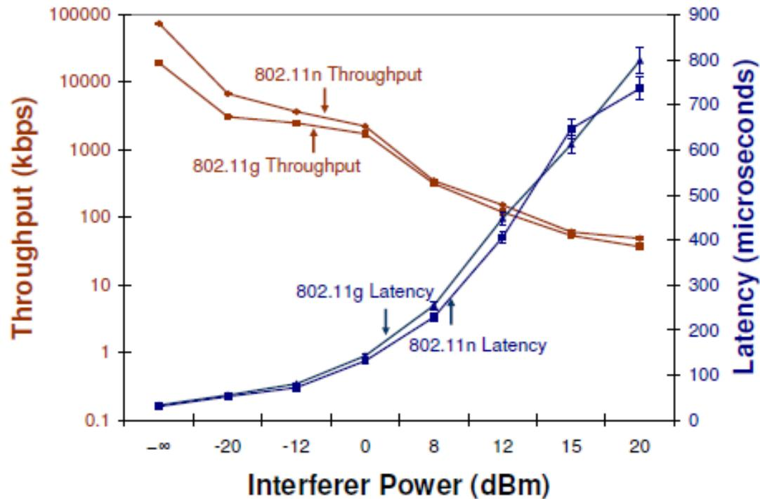
*Throughput and latency vs. interferer power for 802.11g/n.*
