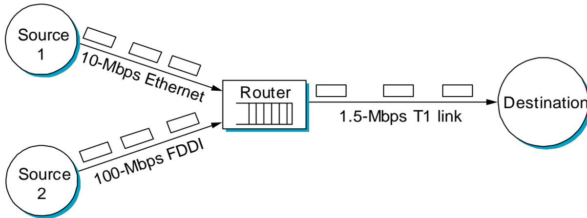
**Figure 6.1 Congestion in a packet-switched network**
