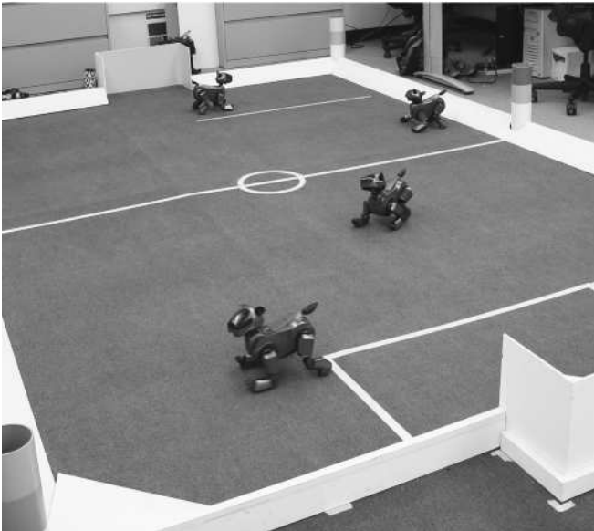
Fig. 1. The training environment. Four robots evaluate different parameter sets simultaneously. The colored markers around the field are used for localization.
