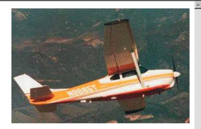
horsepower. In its first model year, which was 1960, the 210 was powered by a 260 horsepower fuel-injected six-cylinder engine that displaced 471 cubic inches. The 210 is the fastest single-engine airplane ever built by Cessna.
