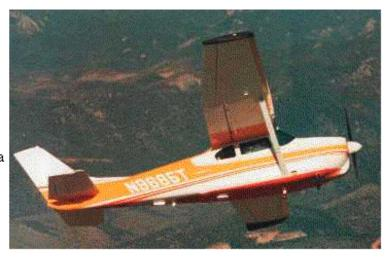
1960, the 210 was powered by a 260 horsepower fuel-injected six-cylinder engine that displaced 471 cubic inches. The 210 is the fastest single-engine airplane ever built by Cessna.
